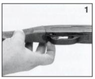
DANGER: The gun will fire when the trigger is pulled intentionally or accidentally when the RED BAND MARKING IS SHOWING.
