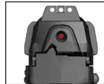
Figure 11 — Firing pin cocked
