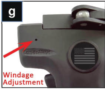
A clockwise turn adjusts the laser to the left
