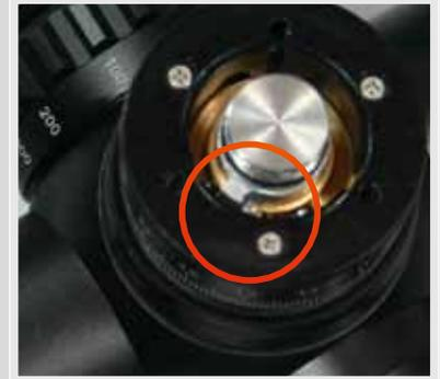
Reinstall the knob and keep in mind to position the two screws at 3 and 6 o'clock. Press the knob firmly against the air resistance on the scope and tighten the screws again.
