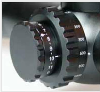
To use the parallax/focus adjustment, rotate the knob on the left side of the adjustment turret until the numeral corresponding to the known target distance lines up with the reference mark. If the distance is unknown, rotate the adjustment knob until the target image is sharply focused.
