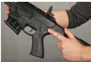
Photo 6-) Push takedown pin at the back side of lower frame receiver by a tool or your finger as in the photo.
