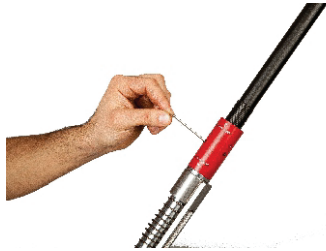
Photo 11-) Unscrew the fixing screws which are on the gas cylinder with 2,5mm allen wrench
