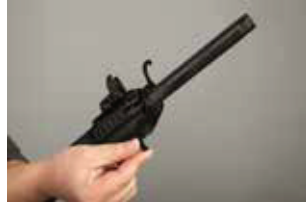
Photo 9-)Use your TR-12 Special Wrench Set for starting to disassemble forend of your shotgun.
