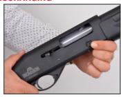
2- Push the bolt release button on the right side of case. Mechanism will slide strongly forward. WARNING!! Be careful not to place your hand thru the way of mechanism while sliding. Keep your hand below as seen in the figure.
