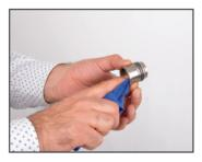
15-Clean the inside and the outer side of the piston with same method. Take care to keep reverse the open sides of rings which are out of the piston.
