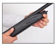
**10-**Loosen the screw in front of the forend to the reverse of clock direction and take off.
