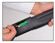
**6-**To discharge the cartridge in the chamber, pull back the bolt hantle.
