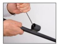
16- Open the holes with a string in the gas room on the bottom of barrel. Clean inside of gas room. Loosen the choke tube and clean the choke and choke bearing. Clean inside of the barrel with a ramrod. Keep quite
