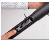
8- Push the carrier at the bottom of the case inside and meantime push the bolt release button once and leave.
