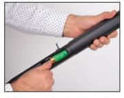
9- Cartridge will drop down to your finger on the carrier. Take off the cartridge. Repeat this operation until the cartridges finish in the magazine.
