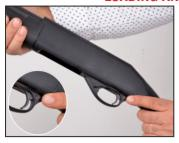
1-Make your shotgun safe by pushing the safety latch on the trigger guide on the left side. Be sure that the RED colour is not seen.
