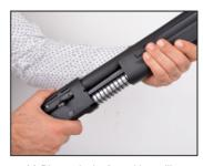
**11-**Dismantle the forend by pulling forward to the barrel end
