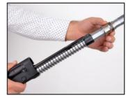
17- To assemble your shotgun again as processes 22,21,20 attach the parts in following order spring, piston and rubber ring. Remember the processes 4,5,6 assembling barrel and forearm.
