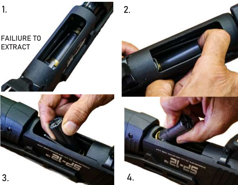
Figure F-2: Clear Double Feed by Rotating Shell Around Lifter
