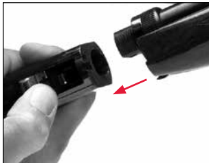
Retract the breech block and insert the barrel into the receiver.
