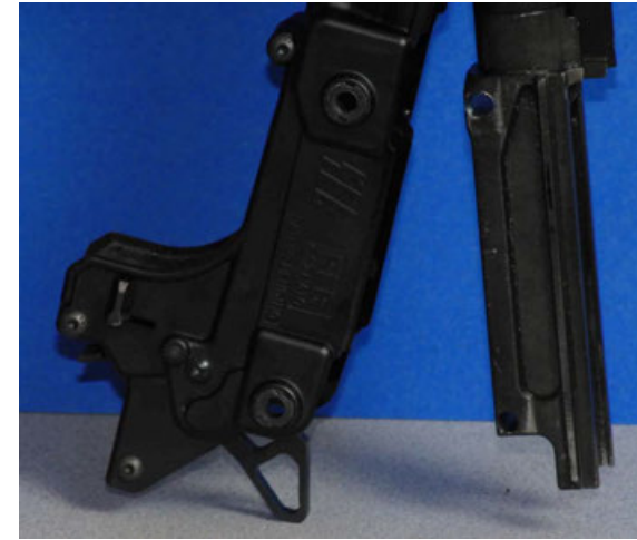
Figure 30: DO NOT rest disassembled rifle on the hammer!
