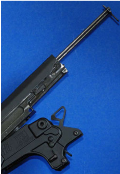
Figure 51: Be sure that the extractors are in the up position and that the rear of the bolt aligns with the carrier before insertion into the receiver
