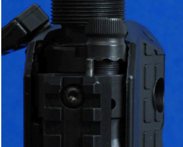
Figure 29: Gas Restrictor Cap set for suppressor use.
