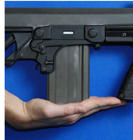
Figure 23:Smack the base of the magazine with the palm of your hand
