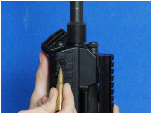
Figure 38: Use the nose of the bullet to push out the forward assembly pin
