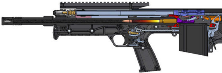
Figure 14: The bullet begins its journey down the bore
