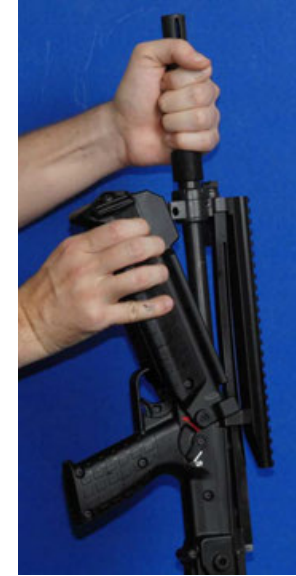
Figure 39: Grasp the barrel with one hand and pull down the handguard
