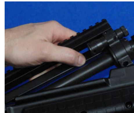
Figure 40: Push the ejection chute on the right side to remove it
