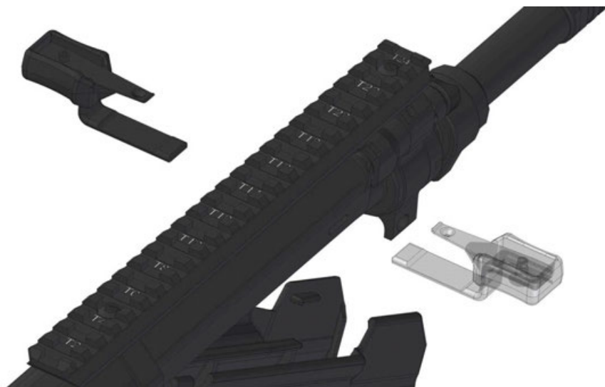
Figure 45: The Charging handle is easily moved to either side
