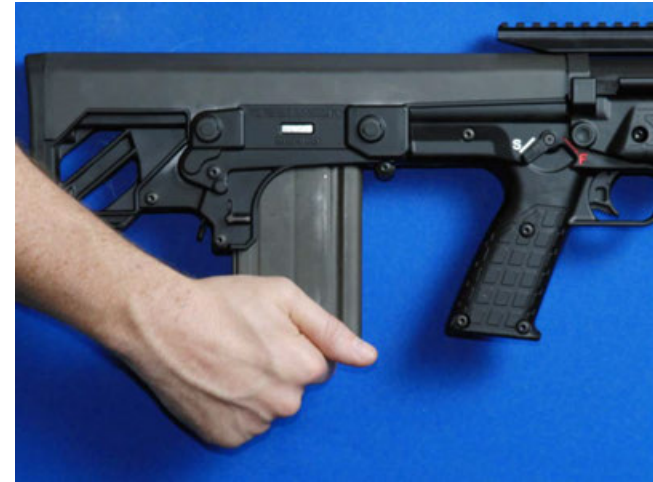
Figure 3: Insert the magazine straight up
