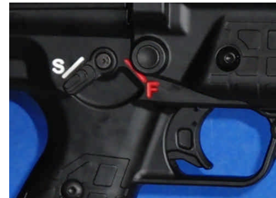
Figure 24: Move the safety selector from Safe to Fire
