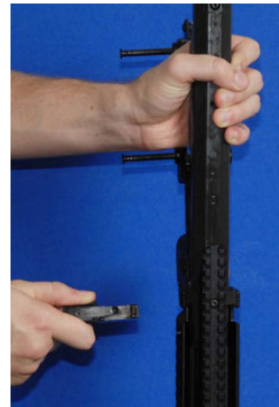
Figure 36: While grasping the carrier and receiver, pull the charging handle straight out to remove it
