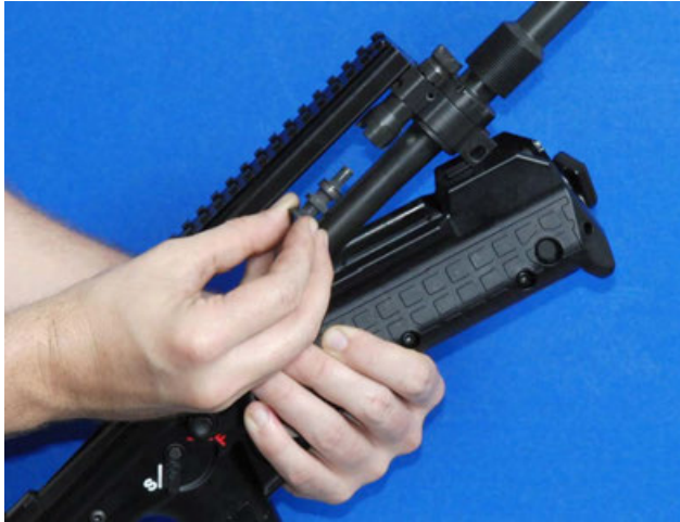
Figure 48: Wiggle the piston to remove
