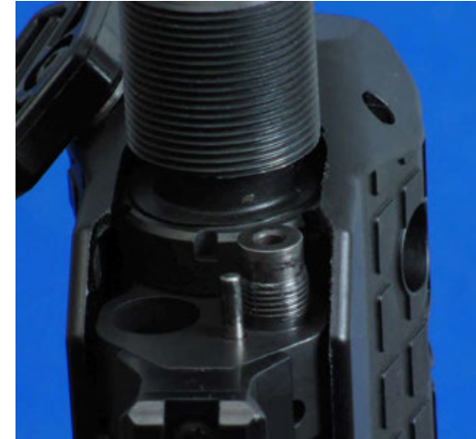
Figure 50: The gas restrictor cap is disassembled and ready to be cleaned
