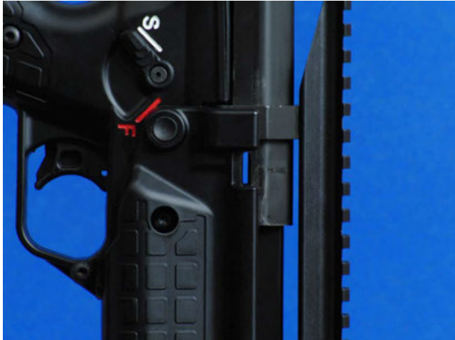
Figure 52: Align the hole on the carrier to the slot in the handguard to reinstall charging handle
