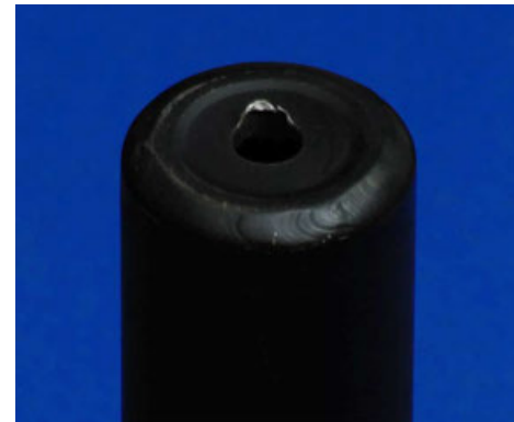
Figure 2: Baffle Strike caused by Subsonic Ammo
