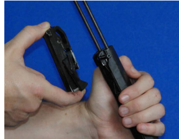
Figure 43: With the pin pushed out, the bolt is easily removed
