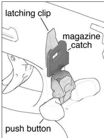
Figure 44 – Diagram of Push Button Parts
