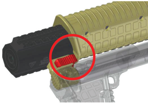
Figure C-7: Rotating Forend latching into the Latch Tab.
